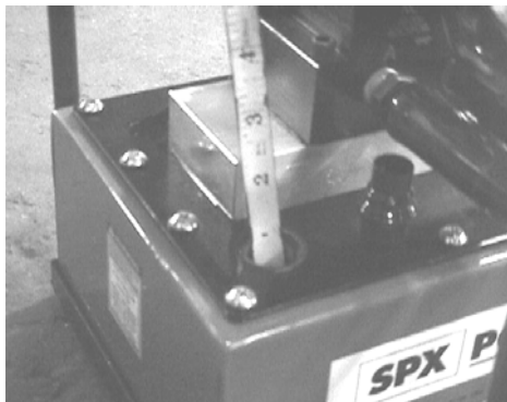
HYDRAULIC PUMP OIL LEVEL
